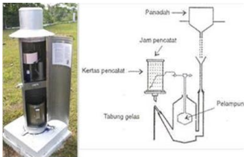
Gambar 1. Automatic Rainfall Recorder (ARR), Type Hilman
